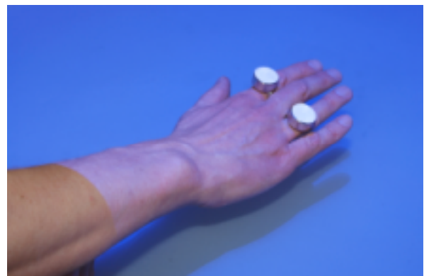
Figure 3 shows a magnetic ring interface worn by the user.
